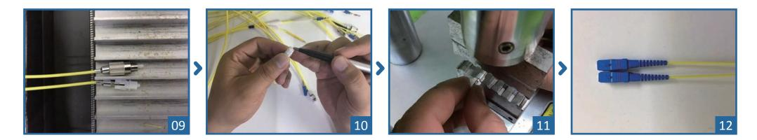
9. When the oven is heated to the proper temperature, the heater light will go off. Place the ferrule into one of the oven's ports. After 20 minutes, remove the connector from the oven and place it in the curing stand to cool. Note: Do not score the fiber before the epoxy is cool and hard.
