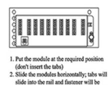
inserted to the rail automatically to lock
