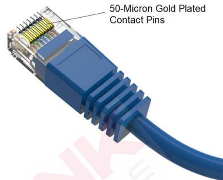
The contact pins of RJ45 plugs used for Ethernet patch cables are gold plated to maintain optimum conductivity with RJ45 jacks (receptacle on the wall). There are several kinds of gold plating thickness available in the market. The lowest grade plating is called flash gold with the thickness at a mere 3 to 6-micron. The highest plating is 50-micron.
