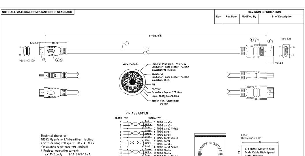
c.2.0~3.0M=2.0mA; d.3.0~5.0M=3.0mA; e.5.0~10M=5.0mA; f.10~15M=7.0mA; 5)Conductive resistance: 4 Ohm Max
