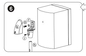
BOSE ACOUSTIMASS LOUDSPEAKERS Attach universal bracket(h) to pole using screw (i)
