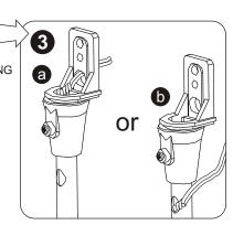
FOR LOUDSPEAKERS WITH THREADED HOLE Secure universal bracket(h)to upright using screw(i). The speaker cable should be Connected to the speaker and threaded through the upright as shown in fig 3a or 3b. The speaker should be fixed to bracket (h) Using washer (r) and either screw(o) or (p) depending on speaker type, Fit cover cap (k) if required.
