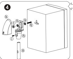
FOR LOUDSPEAKERS WITH KEYHOLE TYPE FIXING Secure universal bracket(h)to upright pole using screw(i). The speaker cable should be threaded through pole and bracket as shown in fig 3a. Or 3b. Assemble thumbnut(t)washers(s)and M4
