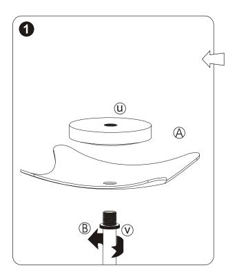
Insert assembled tube (B) into base (A) and screw
