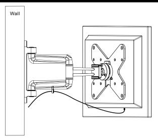
Connect cables to your TV and run cables through the wire clip. **Note:** Leave slack in cable for arm movement.
