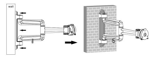
Install the decorative covers along wall plate rail until they fit onto the wall plate.
