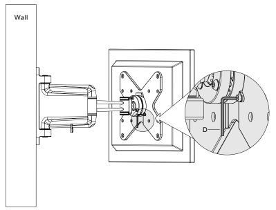
Carefully lift your TV and hook VESA plate onto the mounted head. Tighten screws (that is previously removed) to secure.
