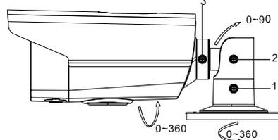
Figure 2-7 3-axis Adjustment
