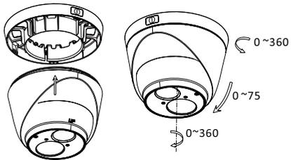
Figure 2-3 3-axis Adjustment
