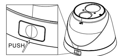
Figure 2-2 Release The Lock Screw
