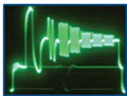
Multiburst Waveform Test
