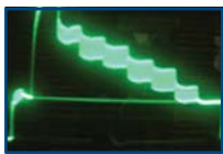
Full Field Color Bar Test: Waveform
