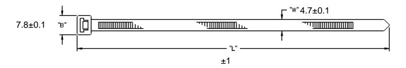
Material: UL Approved Nylon 66/94V-2, corrosion resistant, well insulation, difficult to aging.
