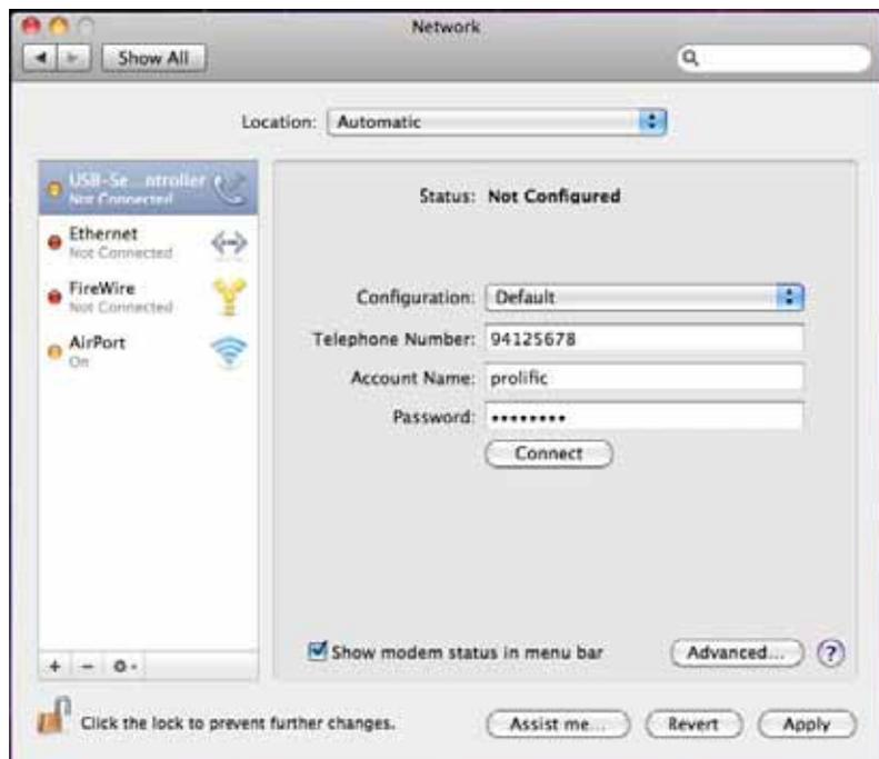
5. You can click on the Advanced button to set the correct modem vendor and model. The default modem settings normally would work on any RS-232 modems.
