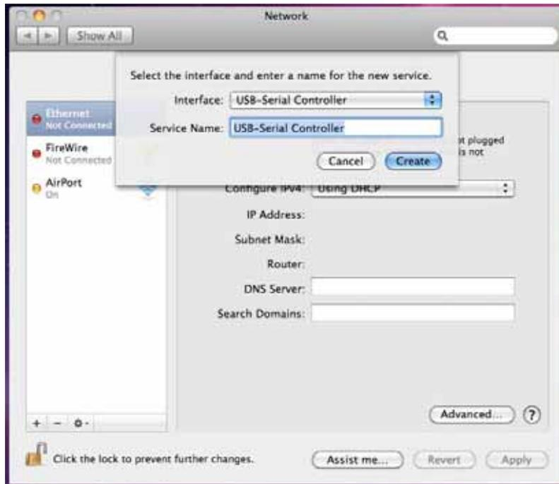
4. Now the “USB-Seruial Controller” device is added to the list and you can start to configure the RS-232 modem Internet dial-up settings attached to the USB to RS-232 adaptor.
